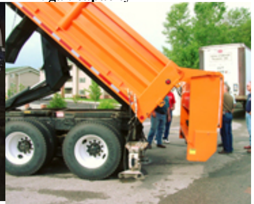
Figure 21. Integrated tailgate 225gal. capacity
